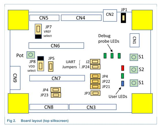
Table 1 below shows the layout of the LPCXpresso804 board, indicating location of jumpers, buttons, connectors/expansion options and MCU devices.
