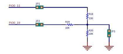
By enabling PIO0\_11 as a DAC output, a test signal can be driven to a circuit probe connected to JP3, then the voltage at the voltage divider formed by R18 and R20 can be measured using an LPC804 ADC input (PIO0\_19). In order to use this circuit it is recommended that R15 is removed and S3 set to the VCC position.
