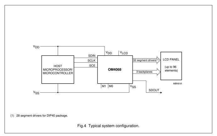
The host microprocessor/microcontroller maintains the 3-line bus communication channel with OM4068. The internal oscillator requires no external components. The appropriate intermediate biasing voltage for the multiplexed LCD waveforms are generated on-chip. The only other connections required to complete the system are to the power supplies (V<sub>SS</sub>, V<sub>DD</sub> and V<sub>LCD</sub>) and suitable capacitors to decouple the V<sub>LCD</sub> and V<sub>DD</sub> pins to V<sub>SS</sub>.
