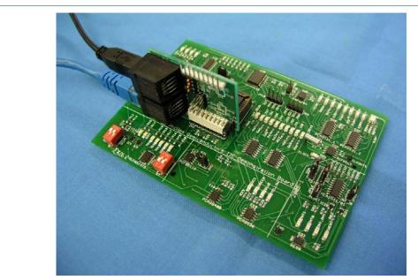
Fig 2. OM6293 fitted to the 9-pin header on OM6275 I2C 2005-1
