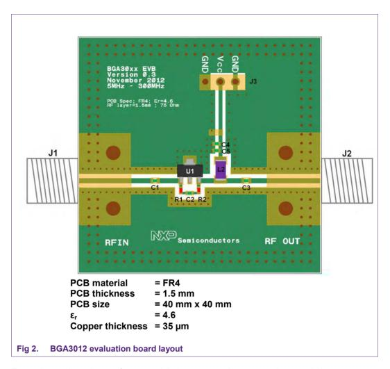
For optimum distortion performance it is important to have enough ground vias underneath and around the MMICs ground pins. This lowers the inductance to the ground plane. The evaluation board is made with two layer FR4 material.
