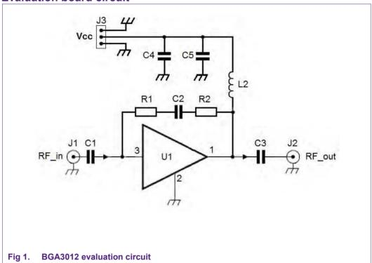
The power supply is applied on the center pin of connector J3 and is applied to the MMIC via choke L2 which provides RF blocking to the supply line. Capacitors C4 and C5 are supply decoupling capacitors.
