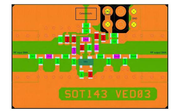
Fig 16. PCB Assembly drawing Amplifier design VED
