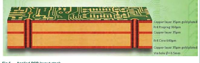
Fig 5. Applied PCB layout stack
