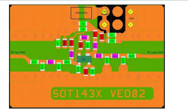
Fig 20. PCB Assembly drawing Amplifier design VED
