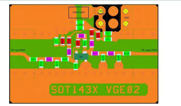
Fig 18. PCB Assembly drawing Amplifier design VGE
