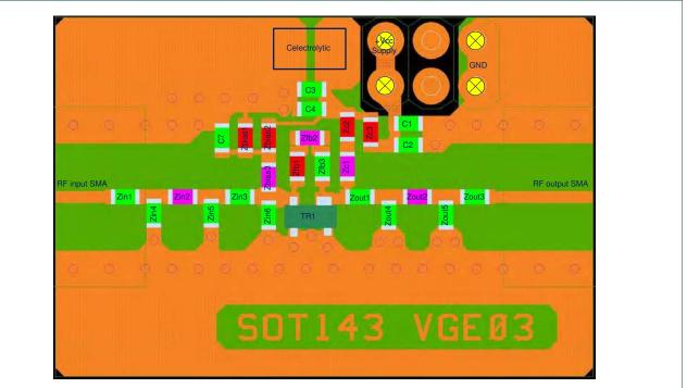
Fig 14. PCB Assembly drawing Amplifier design VGE
