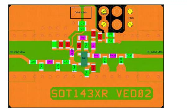
Fig 26. PCB Assembly drawing Amplifier design VED
