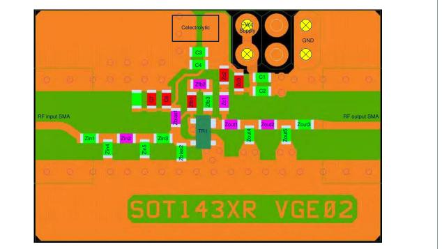
Fig 24. PCB Assembly drawing Amplifier design VGE
