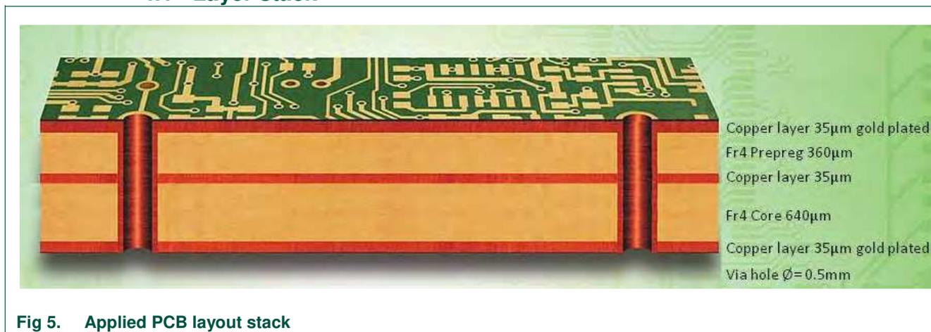
Fig 5. Applied PCB layout stack
