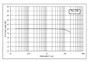
Fig.14 Voltage gain - Frequency
