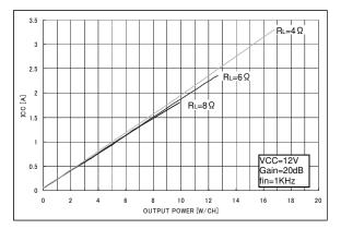
Fig.4 Current consumption - Output power
