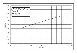
Fig.1 Current consumption - Power supply voltage
