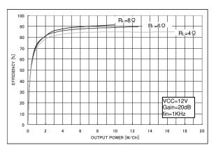
Fig.3 Efficiency - Output power
