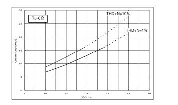
Fig.9 Output power – Power supply voltage
