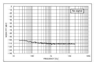
Fig.19 FFT of output noise voltage
