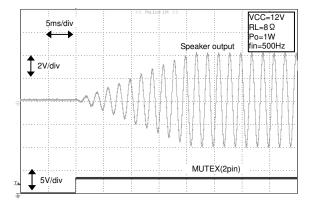
Fig.5 Wave form when releasing soft-mute
