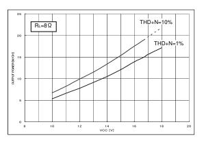
Fig.7 Output power – Power supply voltage
