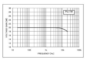
Fig.20 Voltage gain - Frequency
