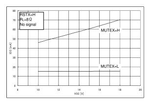
Fig.2 Current consumption - Power supply voltage
