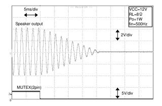
Fig.6 Wave form when activating soft-mute
