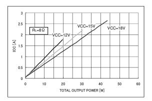
Fig.8 Current consumption - Output power
