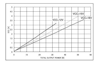
Fig.12 Current consumption - Output power
