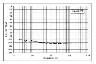
Fig.13 FFT of output noise voltage
