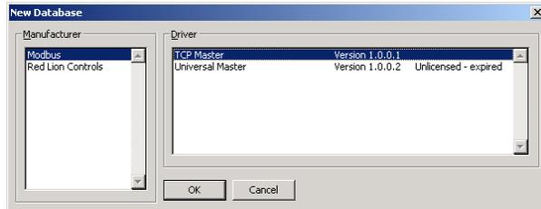
Select the appropriate manufacturer and driver, and press the OK button to close the dialog box. The server will then be configured to use the appropriate protocol, and a single device icon will be created in the left-hand pane.
