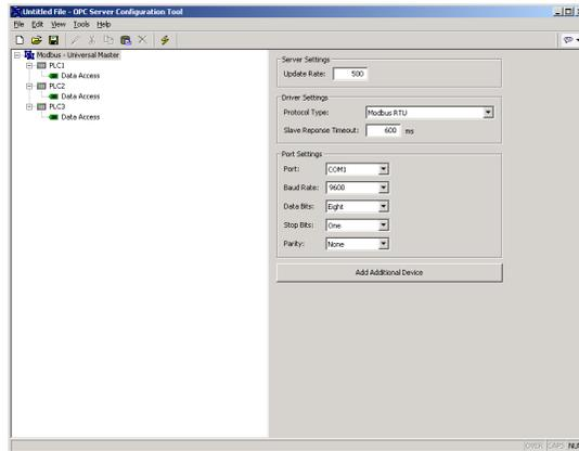
In the example above, the Modbus Universal Master protocol has been selected, and two additional devices have been created, indicating that a total of three remote devices are to be accessed. The right-hand pane of the window shows the properties of a single device. Note that the devices are given default names by OPCWorx when they are created. These names may be changed by selecting the appropriate icon in the left-hand pane, and simply typing the new device name.
