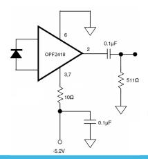
Note that the 10W resistor and bypass capacitor are critical.
