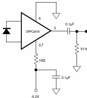
Note that the 10W resistor and bypass capacitor are critical.
