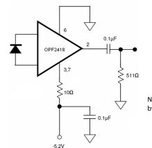
Note that the 10W resistor and bypass capacitor are critical.
