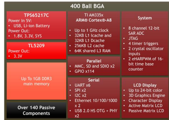
Figure 0.1. OSD335X Block Diagram
