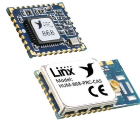
Figure 9: Standard (top) and Pre-certified (bottom) HumPRC™ Modules
