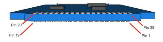
mangOH<sup>™</sup> PCB physical pinout
