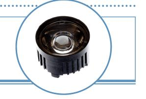
These water-clear polycarbonate lenses with black holders are specifically designed to mate with Optek's 6x6mm power surface mount LEDs (OVSxxxCR4 Series) to provide a more narrow beam angle. Lenses are available in both 15° and 23° viewing angles. The lenses and holders sit firmly over the LED component and is easily attached to the PCB/MCPCB with adhesive.
