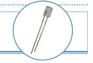
The **OVLLx8C7** series is designed for superior performance in signage and lighting applications that require wide-angle uniform light output. These devices combine a high-intensity LED with a unique flat-topped T-1¾ package to provide both high brightness and a wide spatial radiation pattern.
