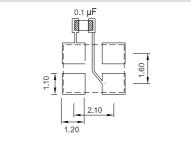
To ensure optimal oscillator performance, place a by-pass capacitor of  $0.1 \mu F$  as close to the part as possible between Vdd and GND pads.
