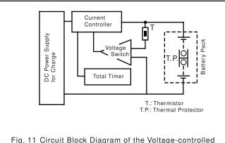
ig. 11 Circuit Block Diagram of the Voltage-controlled Charge System
