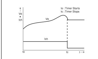
Fig. 3 Charge Characteristics of the Timer-controlled Charge System
