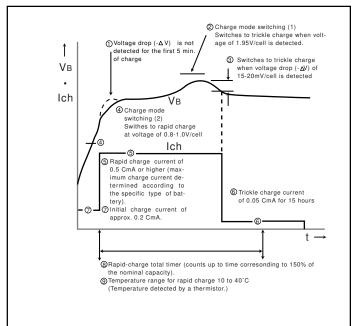
Fig. 6 Typical - $\Delta V$  Cut-off Charge System
