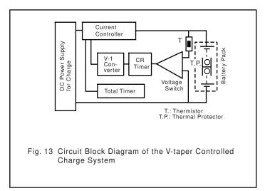
rapid charge current is supplied as a tapered current, decreased at a predetermined rate over a predetermined length of time, and then switched to trickle current. Supplying the decreasing taper current makes it possible to achieve a higher charge level than with the voltage-controlled charge system.
