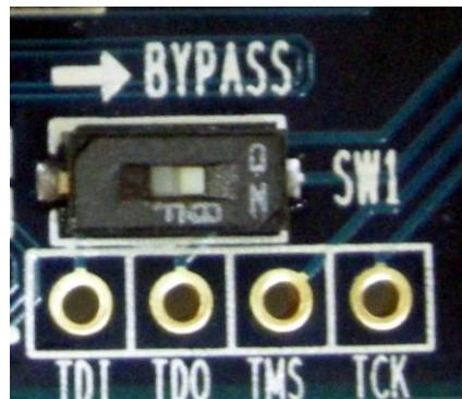
Figure 3.6 The JTAG Switch in “ON” position
