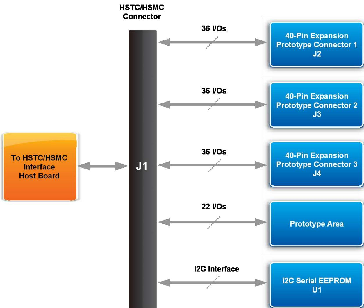
Figure 2.4. The block diagram of the THDB-HTG board
