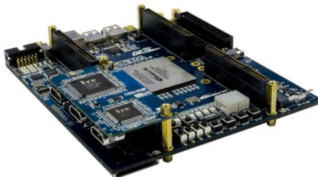
Figure 1-2 Connect HDMI daughter board to DE3 board
