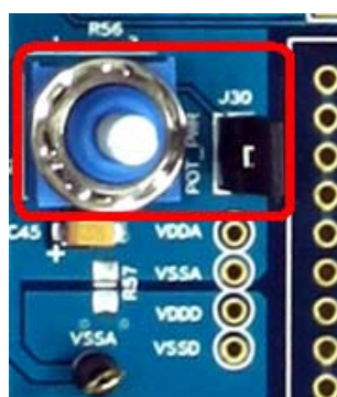
Figure 4-7 CY8CKIT-030 PSoC 3 DVK Potentiometer Power
