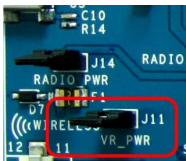
Figure 4-5 CY8CKIT-001 PSoC DVK VR_POWER Jumper
