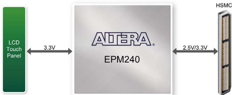
Figure 3-6 Block Diagram of the Bus Controller
