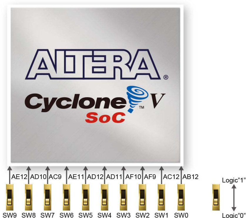
Figure 3-16 Connections between the slide switches and the Cyclone V SoC FPGA
