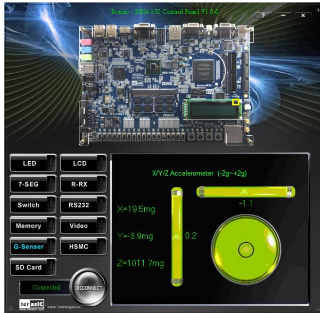
Figure 2-13 Testing the G-sensor
