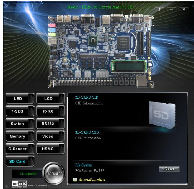
Figure 2-8 Reading the SD Card Identification and Specification
