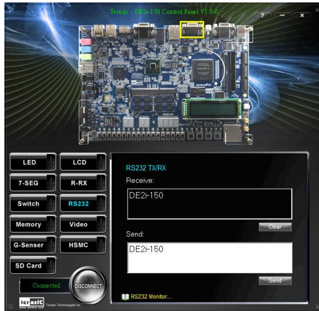
Figure 2-9 RS-232 Serial Communication
