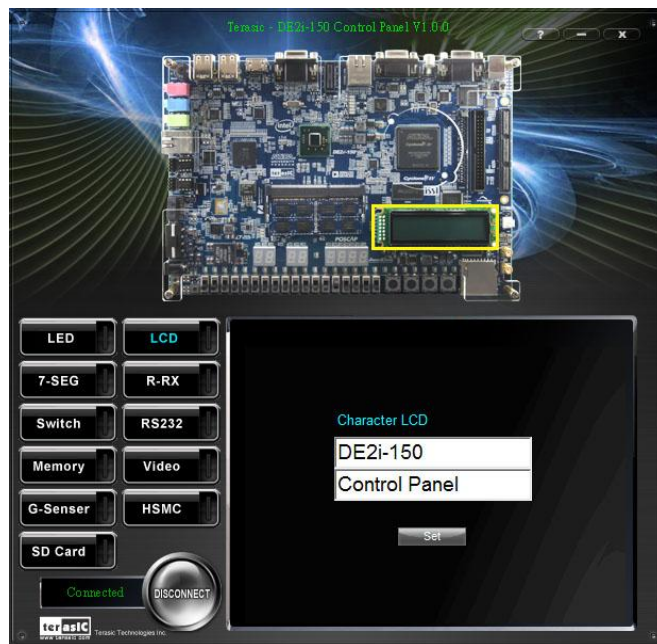
Figure 2-5 Controlling the LCD display
