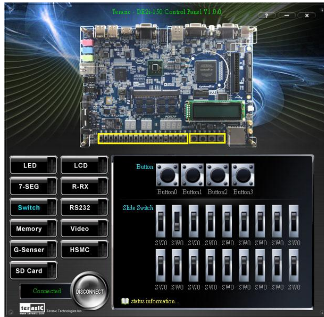
Figure 2-6 Monitoring switches and buttons
