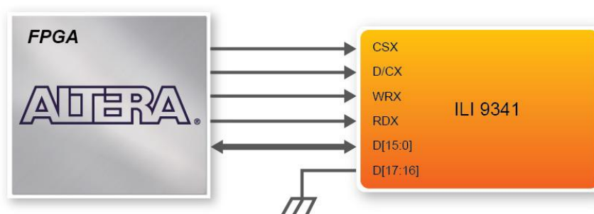
Figure 3-2 Signals of LCD driver connected to FPGA
