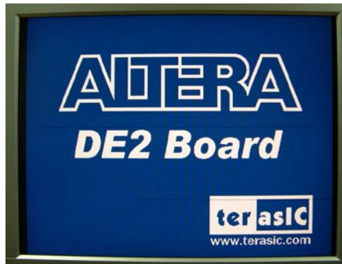
Figure 2.3. The default VGA output pattern.
