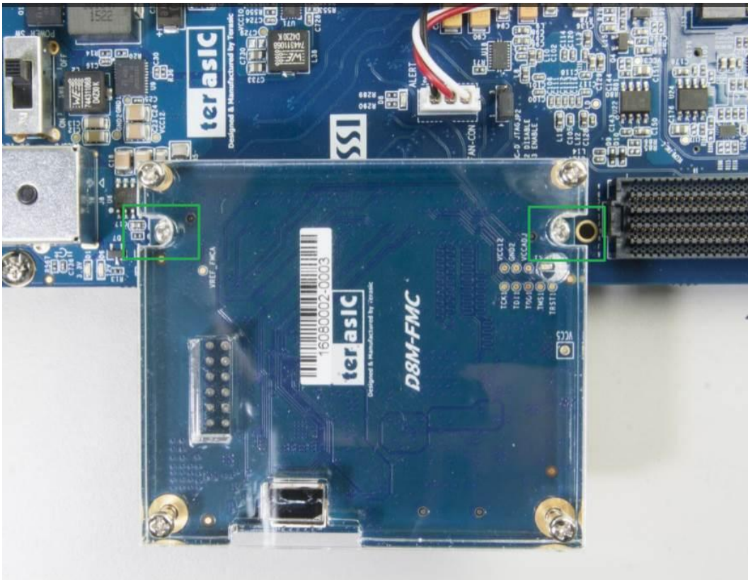
Figure 1-8 demonstrates of how the D8M-FMC will look once installed on the TR5
