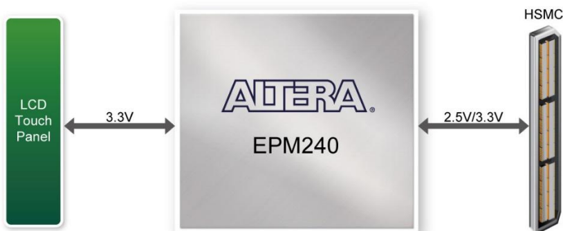
Figure 3-6 Block Diagram of the Bus Controller
