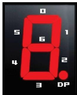
Figure 2-8 Position and index of each segment in a 7-segment display
