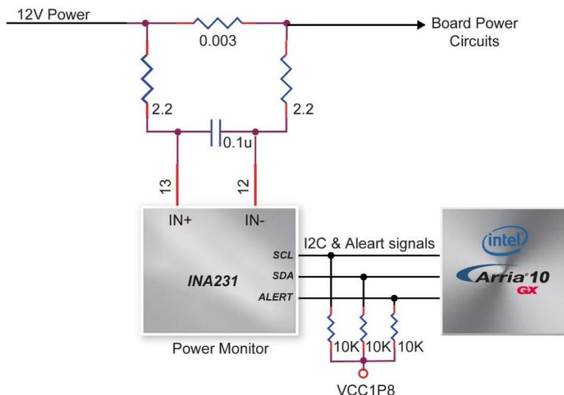
**Figure 2-11** Connections between the Power Monitor and FPGA
