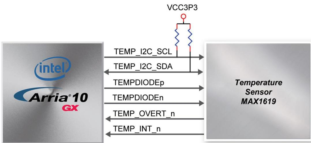
**Figure 2-9 Connections between the temperature sensor and FPGA**
