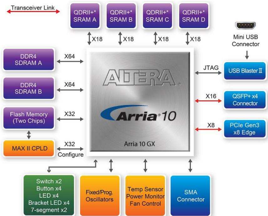
\*Cypress QDRII+ SRAM or functional compatible SRAMs provided by GSI (SigmaQuad-II+) and ISSI (QUADP).
