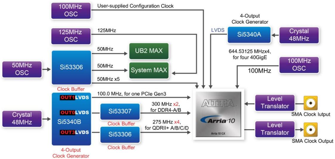
**Figure 2-12 Clock circuit of the FPGA Board**
