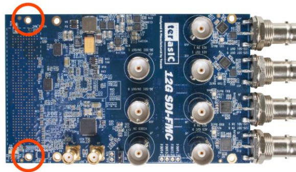
Figure 1-2 Two screw holes on the FMC side of the SDI-FMC
