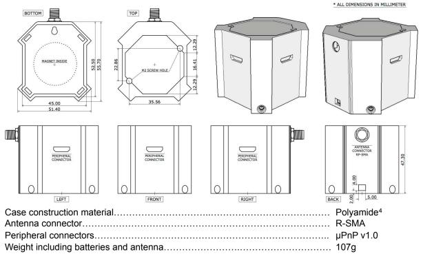
**NOTE:** Peripheral connectors resemble mini HDMI sockets, but they are in no way compatible. The connection of a HDMI device to a peripheral connector may result in damage to one or both devices.
