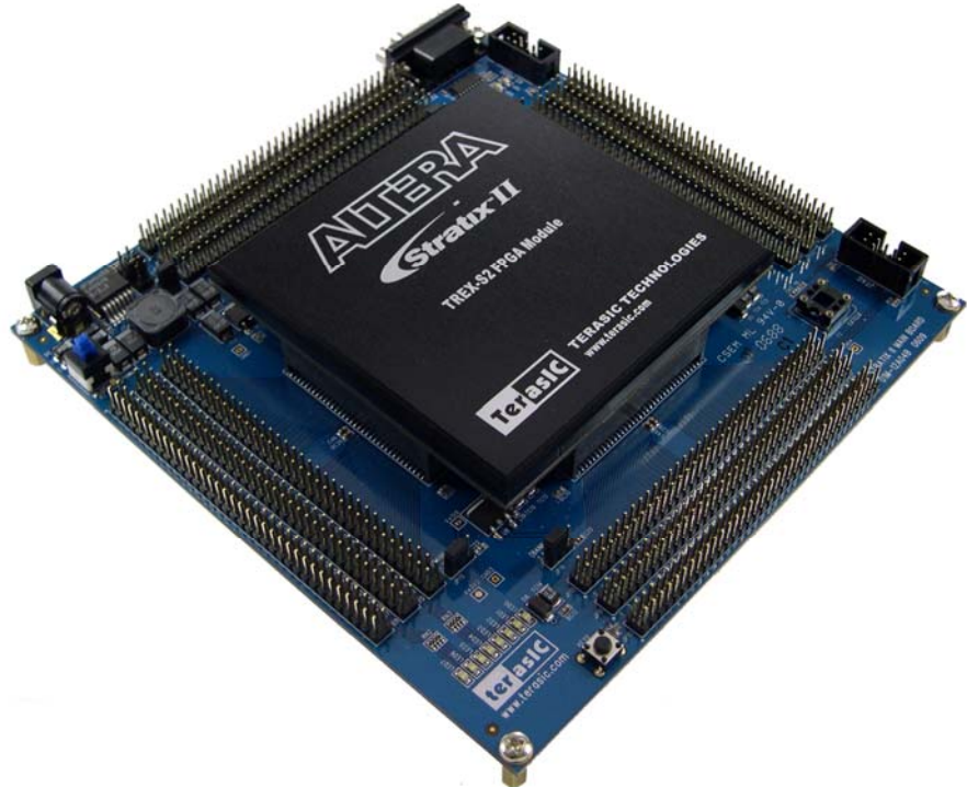
Figure 1.2. TREX-S2 FPGA module plugged onto the TREX-S2-TMA motherboard
