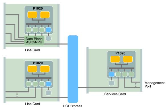
Figure 1. Integrated Dual-Core Device Application
