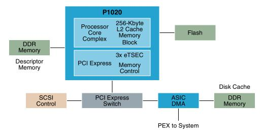
Figure 3. RAID Controller Application Using P1020
