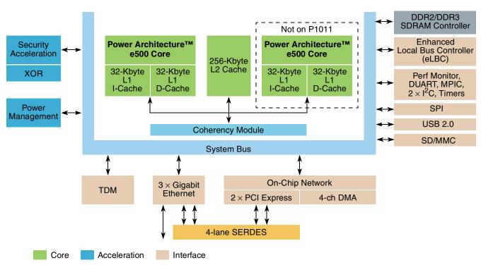
Figure 6. P1020/P1011 Block Diagram
