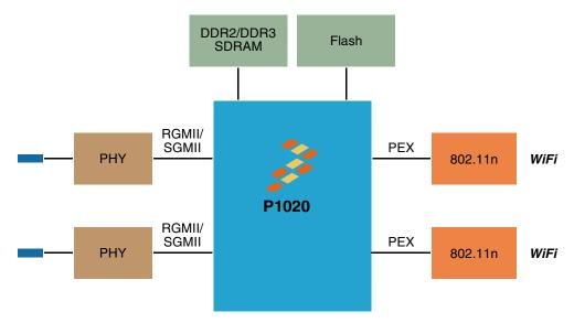
Figure 5. P1020 WLAN Access Point Example
