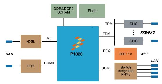
Figure 4. P1020 SMB Multiservice Gateway Example
