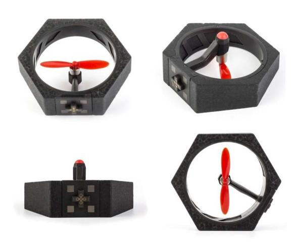
Functions: Airblock power module, install onto main control module position 1 under aircraft mode, the LED turns red to show the head of the aircraft.
