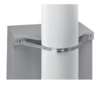
Enable COMLINETM, CONCEPTTM, ACCESSPLUSTM, D-BOXTM and L-BOXTM enclosures to be mounted to poles of various sizes and shapes. Simply attach the galvanized steel channel bar to the mounting holes at the back of the enclosure, then wrap the stainless steel strap around the pole and through the bar. Kit includes two mounting channels, two straps suitable for up to 12-in. diameter pole, and mounting hardware.
