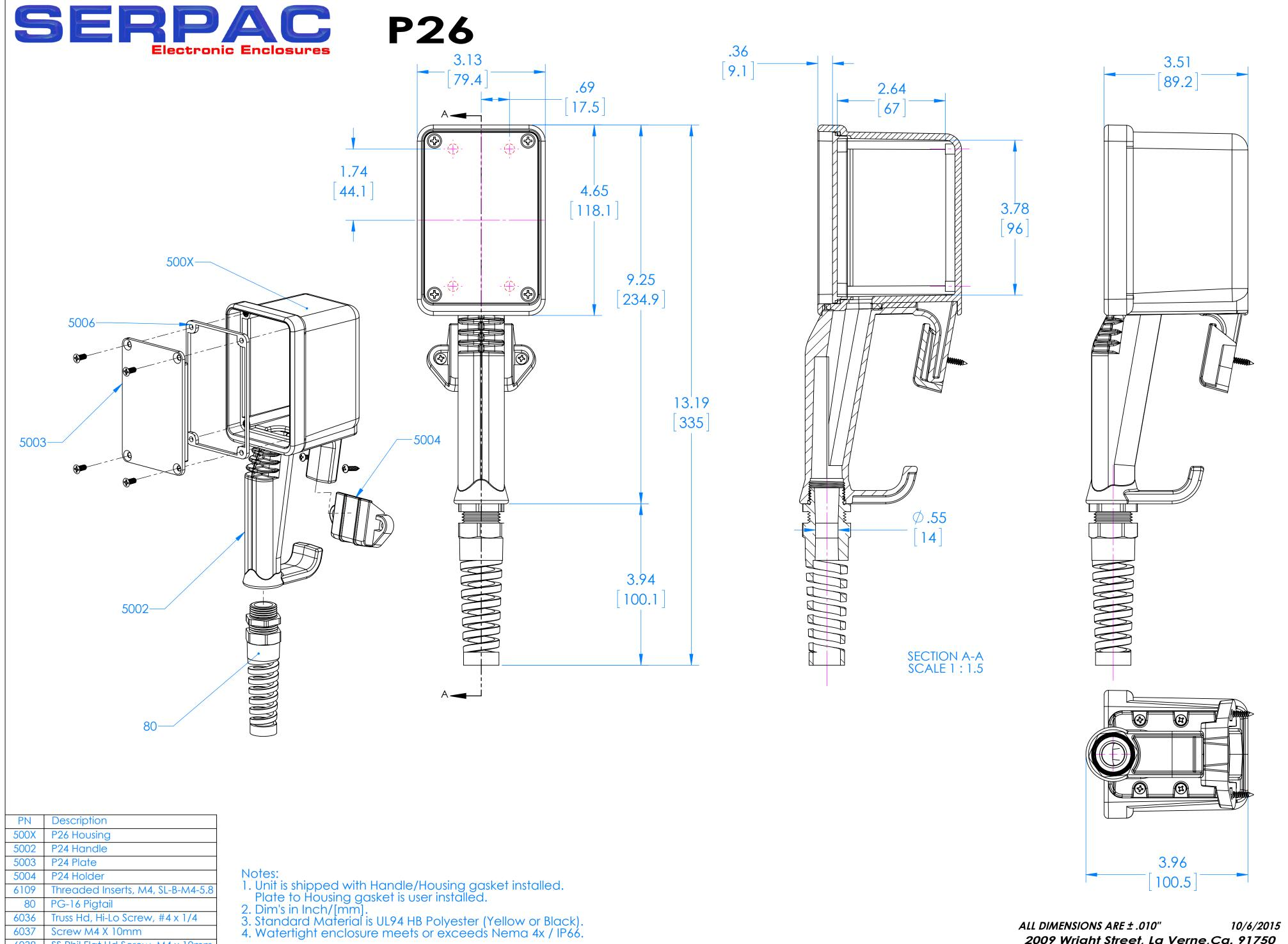
PG-16 Pigtail 80 Truss Hd, Hi-Lo Screw, #4 x 1/4 6036 Screw M4 X 10mm 6037 6038 SS Phil Flat Hd Screw, M4 x 10mm P24 Gasket 8010
