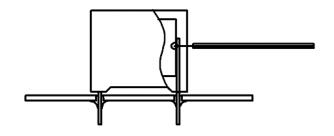
Temperature monitored inside the capacitor.
