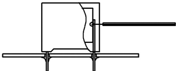
Temperature monitored inside the capacitor.
