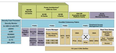
Core Complex (CPU, L2 and Frontside CoreNet Platform Cache)
