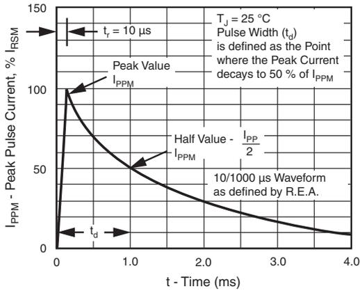
Fig. 3 - Pulse Waveform
