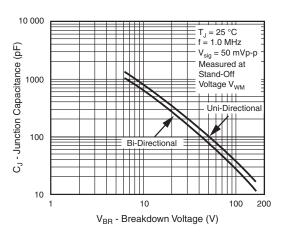
Fig. 4 - Typical Junction Capacitance
