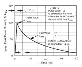
Fig. 3 - Pulse Waveform
