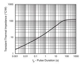
Fig. 5 - Typical Transient Thermal Impedance
