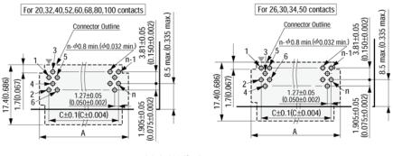
$\ensuremath{\triangledown}$  =Polarity identification Recommended PCB Thickness t=1.6±0.19(0.063±0.007) "n" is number of contacts.
