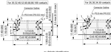
▼ =Polarity identification Recommended PCB Thickness t=1.6±0.19(0.063±0.007) "n" is number of contacts.
