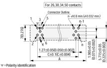
Recommended PCB Thickness  $t=1.6\pm0.19(0.063\pm0.007)$  "n" is number of contacts.
