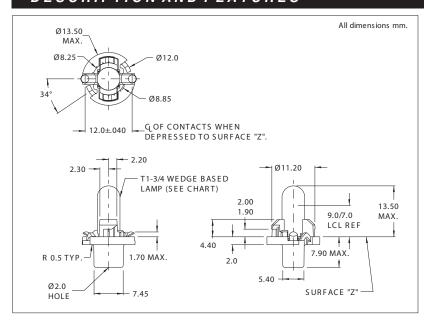
Mounting: Printed circuit board, twist-in
