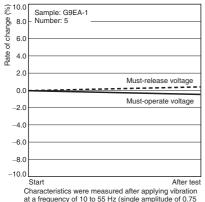
Characteristics were measured after applying vibration at a frequency of 10 to 55 Hz (single amplitude of 0.75 mm) to the test piece (not energized) for 2 hours each in 3 directions. The percentage rate of change is the average value for all of the samples
