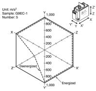
The value at which malfunction occurred was measured after applying shock to the test piece 3 times each in 6 directions along 3 axes.
