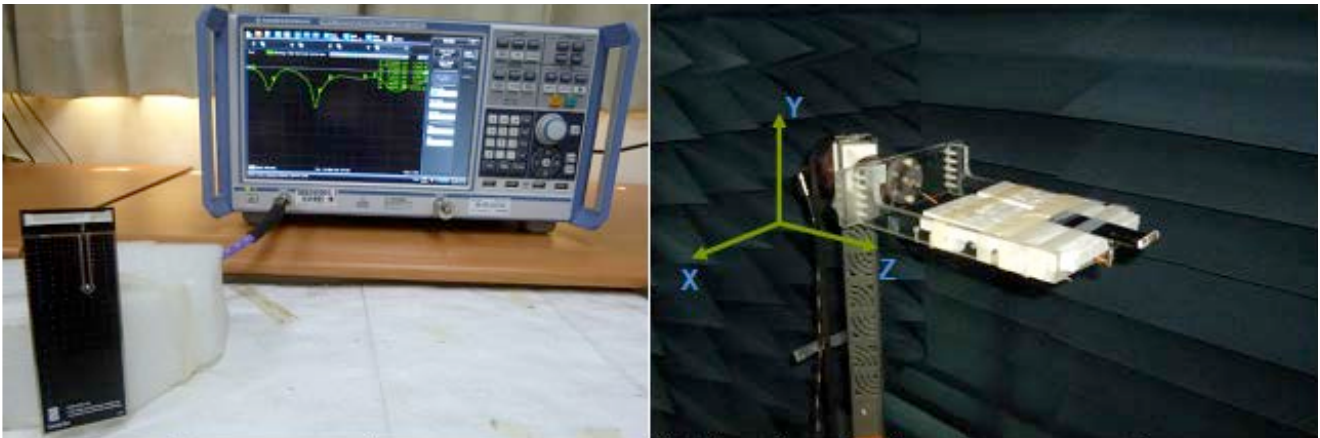
Figure 1. Impedance measurements (left hand) and peak gain, average gain, efficiency and radiation pattern measurements (right hand)
