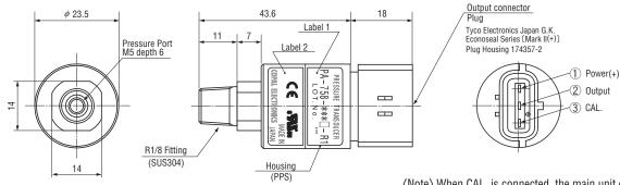
(Note) When CAL. is connected, the main unit of the sensor might malfunction or be damaged.
