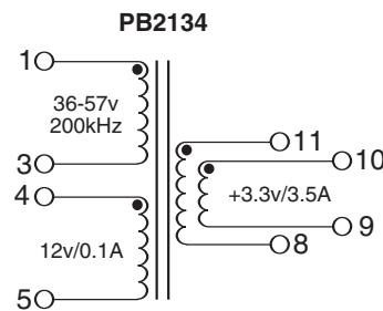
**NOTE:** Pins 10 & 11, Pins 8 & 9 to be connected on customer PCB
