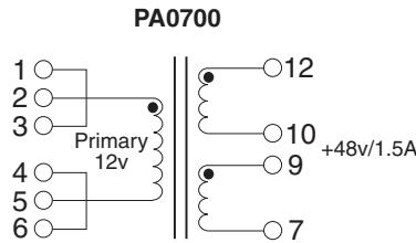
**NOTE:** Pins 9 and 10 to be connected on customer PCB
