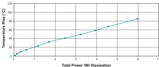
Total Power Dissipation (W) = .001 \* (DCRprimary \* IRMs primary² + DCRsecondary \* IRMs secondary²) + Core Loss (W)
